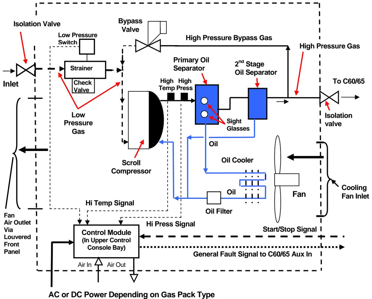
Figure 2. Gas Pack Block Diagram and Flow Schematic
