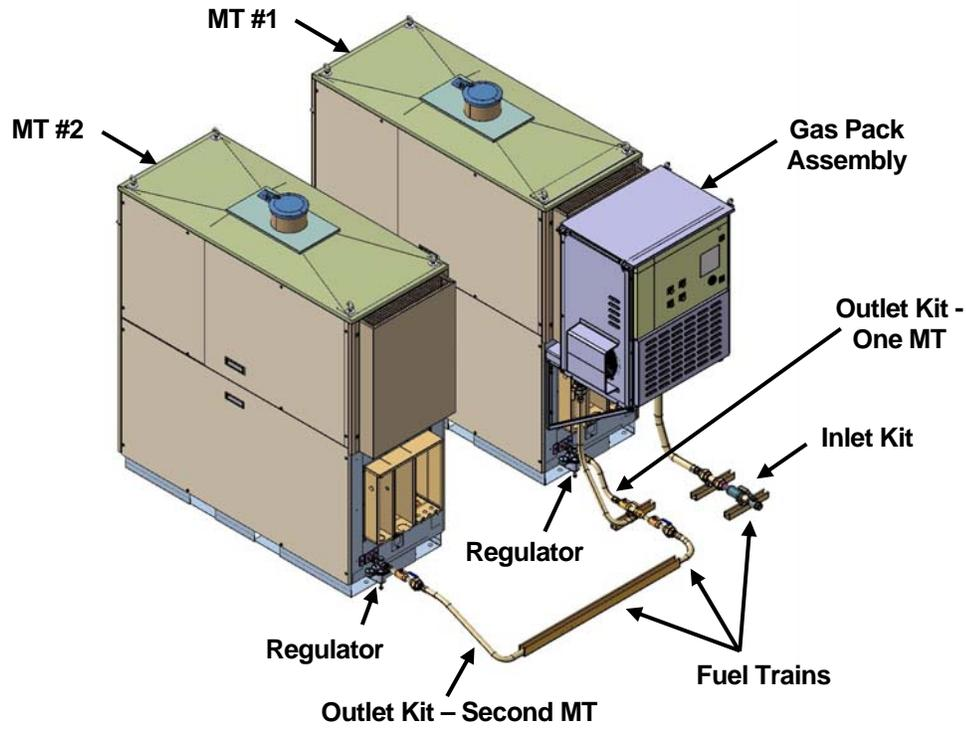
**Figure 3. Installation Overview of 2 MicroTurbines, Gas Pack & Fuel Trains**
