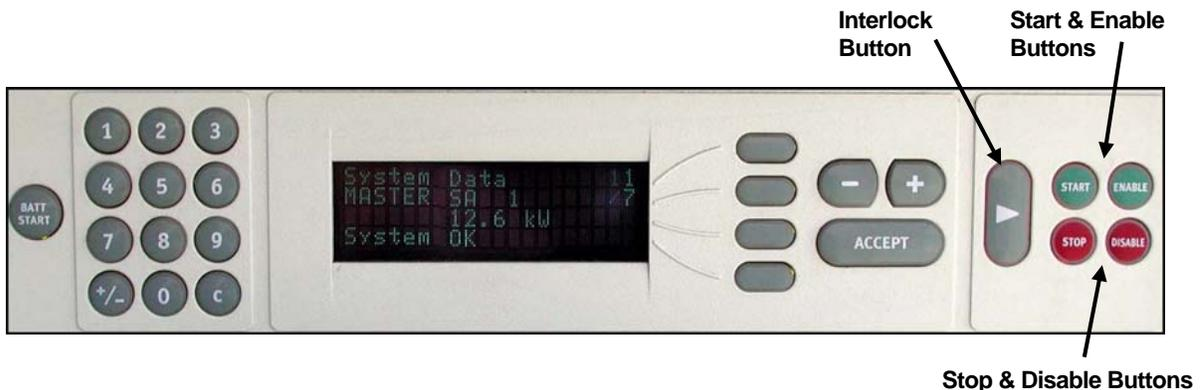
**Figure 8. MT Display Panel and Applicable Functions**
