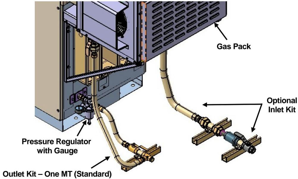
Figure 5. Single MT Installation Showing Gas Pack and Fuel Trains
