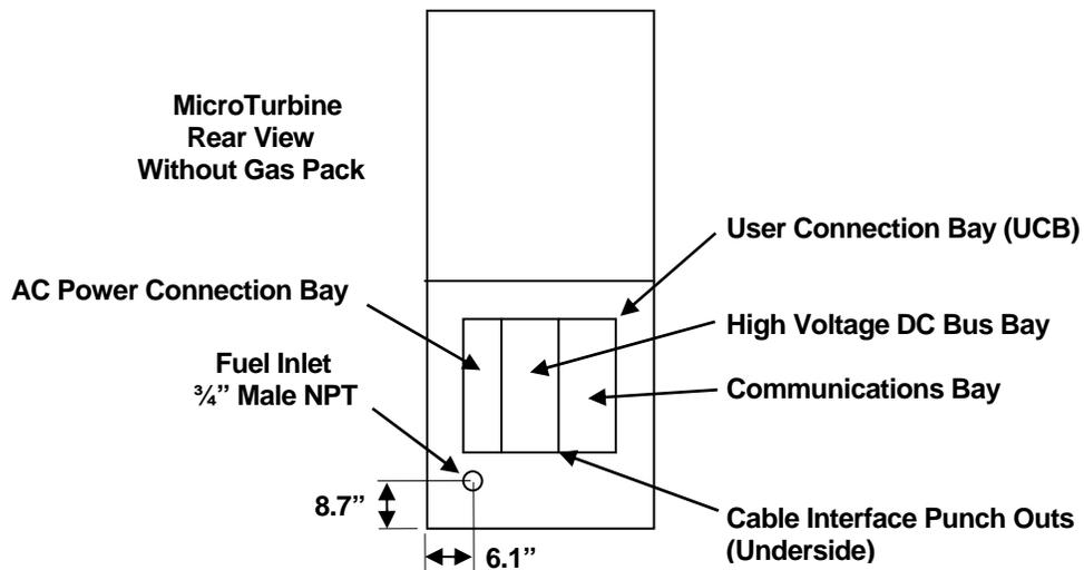
**Figure 4. Rear View of MT Showing High Pressure Fuel Inlet Fitting**
