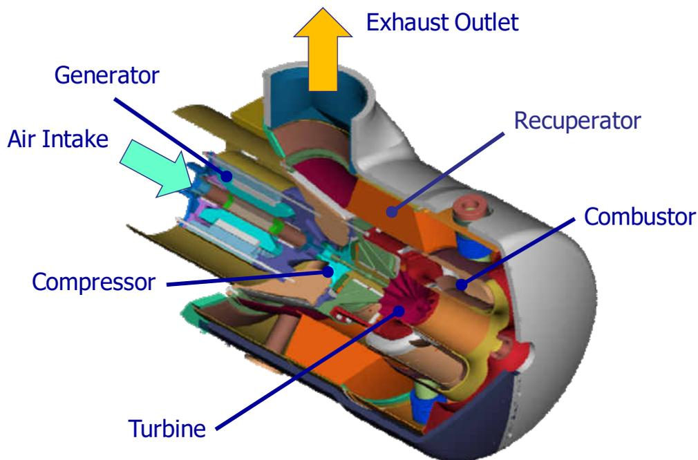
**Figure 2 Cutaway View of a Capstone Microturbine Generator**
