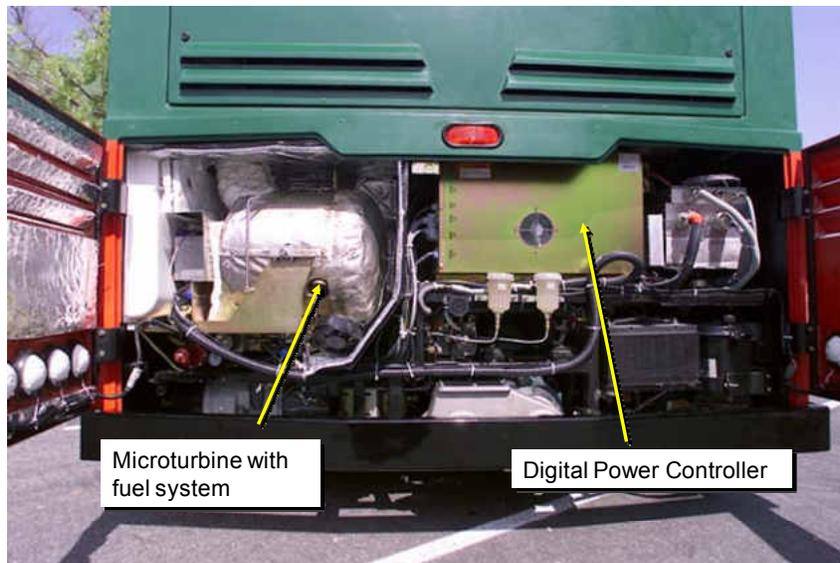
**Figure 4 Capstone C30 Mounted in a Transit Bus**
