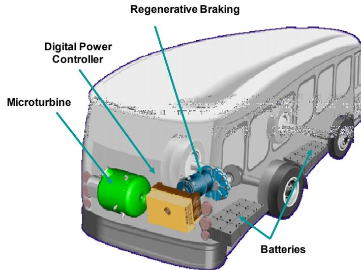
Figure 3 Series Hybrid Electric Drive System
