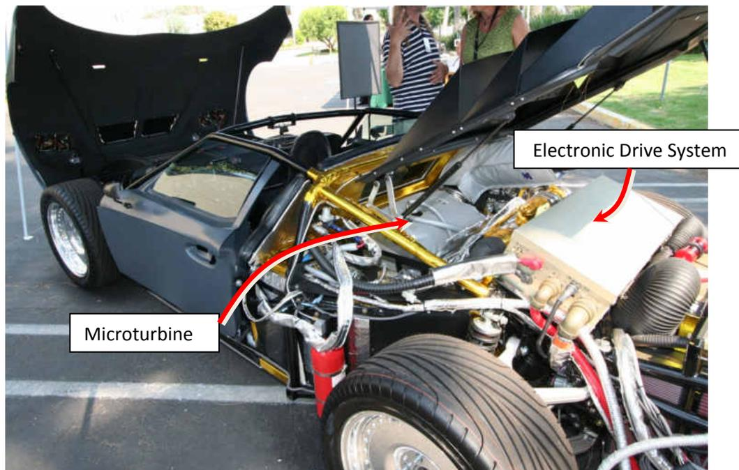
**Figure 11 CMT-380 Microturbine Supercar Concept Vehicle with 30kW Microturbine**
