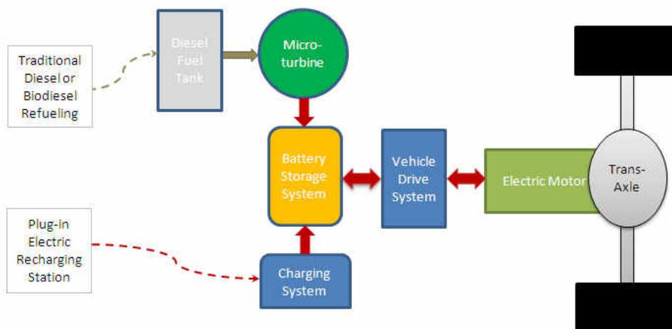
Figure 1 Schematic of a Plug-in Hybrid Electric Drive System
