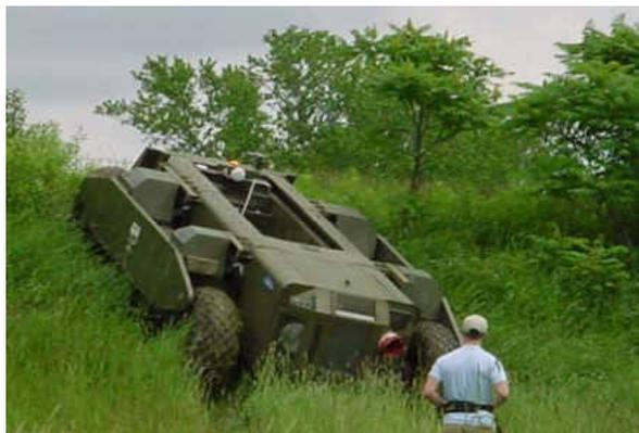
Figure 9 “Spinner” Unmanned Military Prototype using Capstone C30
